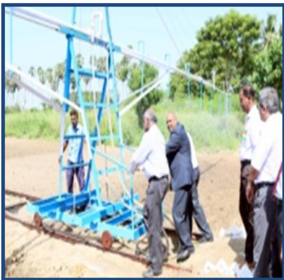
TANUVAS – ILFC – MOVABLE MULTIPLE SPRINKLERS SYSTEM
