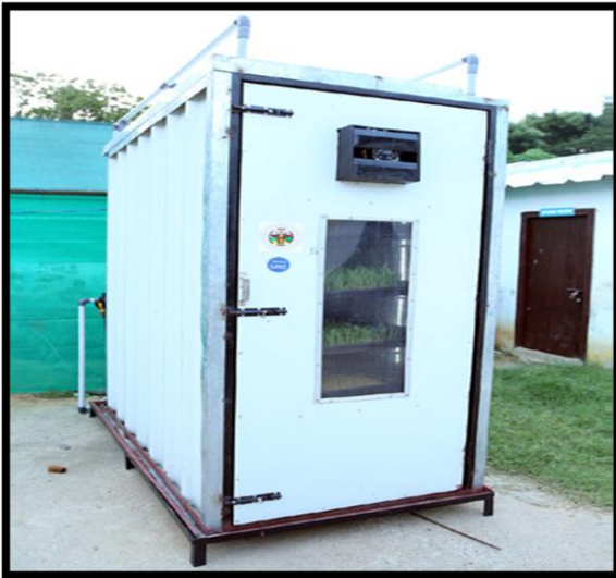
TANUVAS – ILFC – LOW COST HYDROPONIC DEVICE (40 KG / DAY)
